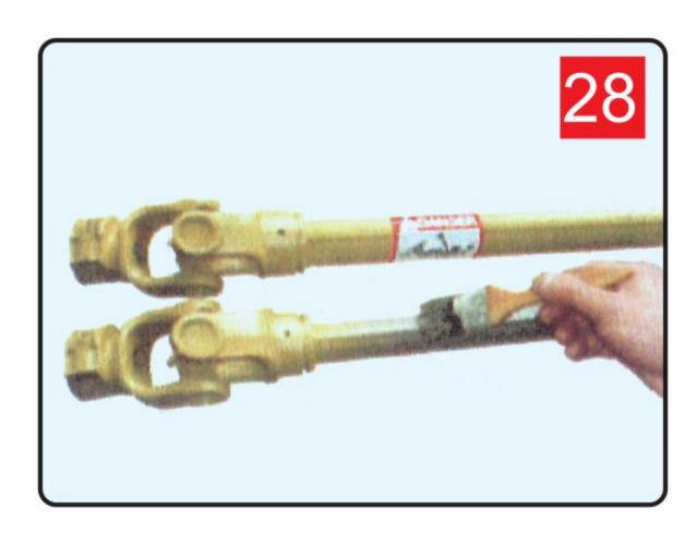
5.Grease the internal drive tube and reassemble the shielding on the driveshaft.
