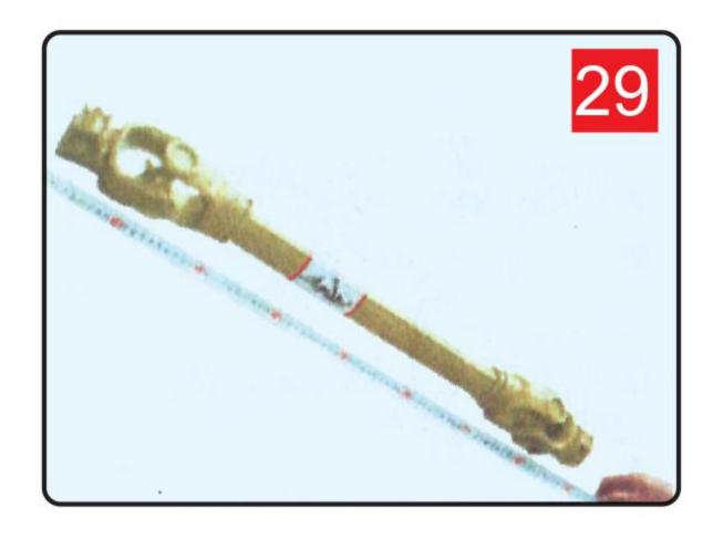
Check the length of the driveshaft in the minimum and maximum positions of the machine. The drive tubes should overlap by 1/3 of their length during working conditions; Shield tubes should never separate while in use.
