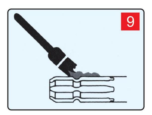
Clean and grease the tractor PTO and implement shaft before installing the driveline.
