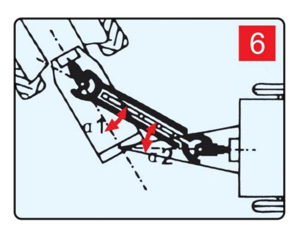
Disengage the PTO if the angles are too large or not identical.
