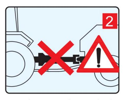
The driveline must be securely attached at both ends. Guards must turn freely on the driveline
