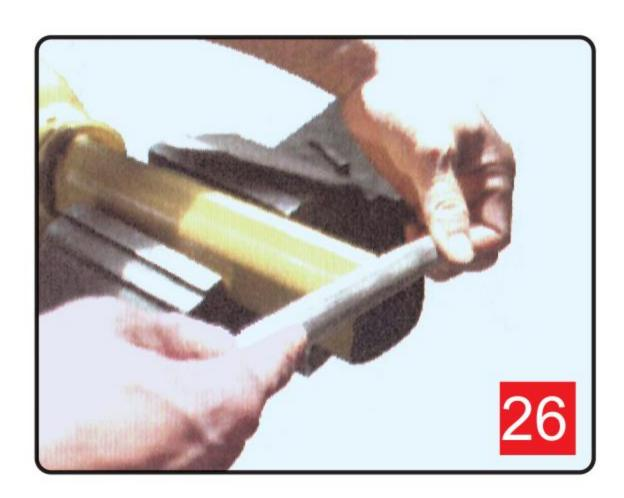
3.Deburr edges of the drive tube with a file and clean all filings from the tubes.
