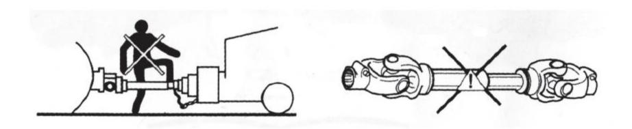
Do not operate the machine without the driveshaft, tractor, and implement shields in place. Driveshaft shields must turn freely on the driveshaft.
