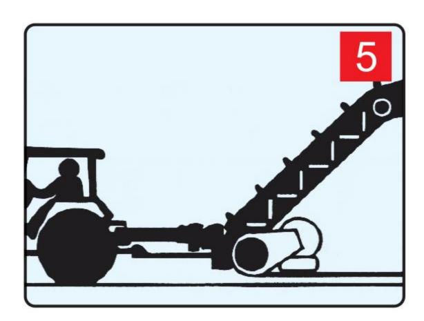
The tractor must be hitched to the implement and positioned so that the angles of the joints are minimal and equal.
