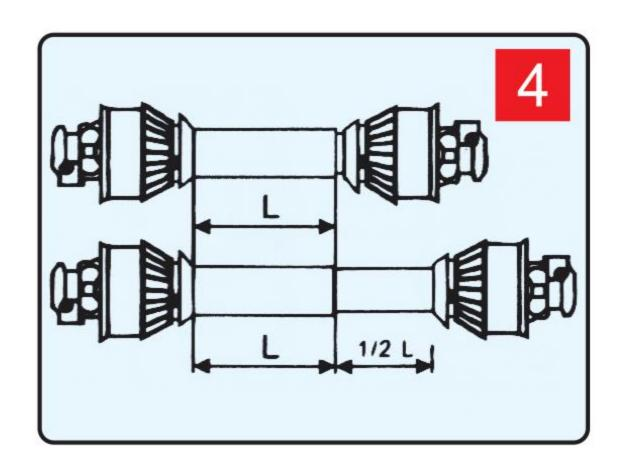
Confirm the minimum and maximum working lengths of the driveshaft.
